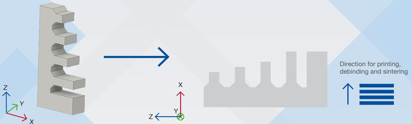
Fig 5: New part orientation for printing, debinding and sintering
