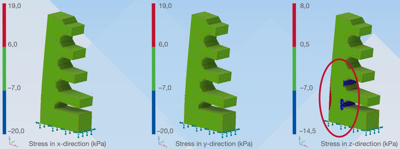
Fig 4: Brown Part Stability in each coordination direction
