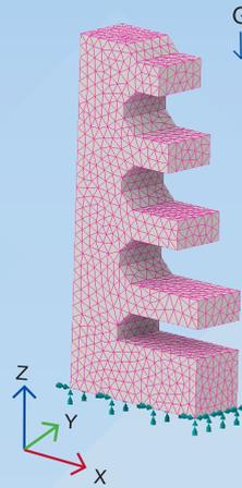
Fig 2: Meshed example part with boundary conditions and gravitational force
