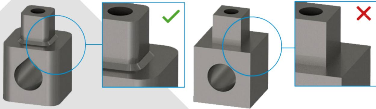
Figure 23: Fillet and Chambers
