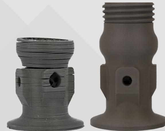
Figure 22: Cooling & Delamination Example
