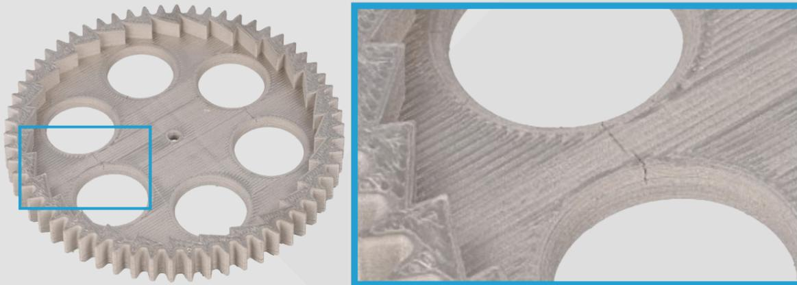
Figure 15: Not Flat & Cracked
