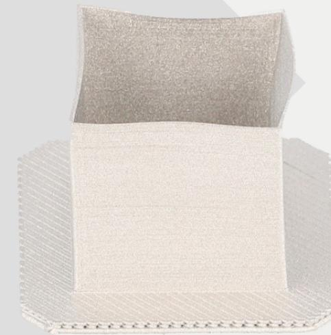
Figure 18: 0.4mm Wall Failure
