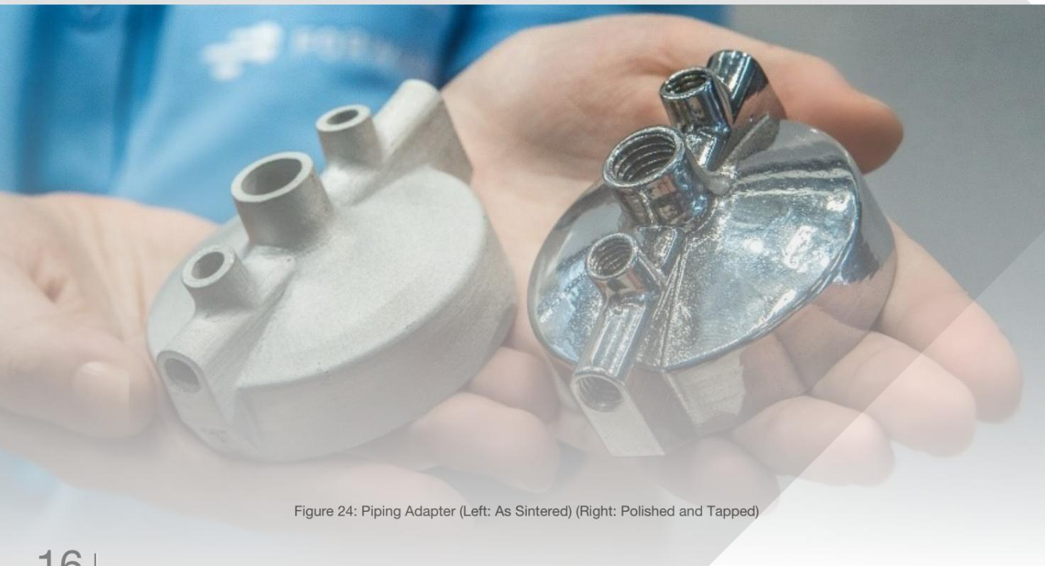
Figure 24: Piping Adapter (Left: As Sintered) (Right: Polished and Tapped)
