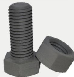
FFF is a manufacturing method in which material is deposited in a series of 2D layers. Multiple layers are stacked on top of each other to create a 3D part. The 3D model in .STL format is cut into several layers or "slices" so that movement instructions, required by the printing system, can be created with Computer Aided Manufacturing (CAM) software, commonly referred to in FFF as a slicer.
