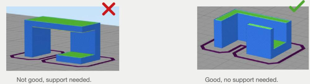
Figure 2 Part Orientation Example
