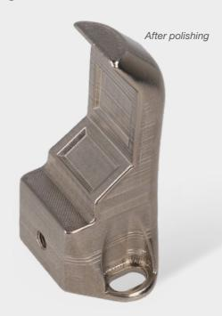
Parts requiring high tolerances may take advantage of traditional metal working methods to produce functional faces. Green state machining enables dramatic reductions in machining costs and capital investment due to Ultrafuse 316L's high machinability in the green state.
