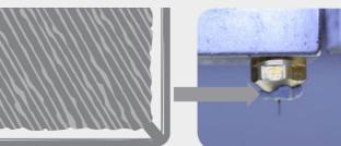
Nozzle is too close to the print bed. The extrudate swells, and the layer is heavily smeared and uneven.
