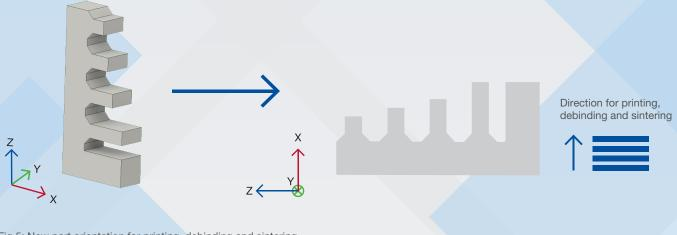
Fig 5: New part orientation for printing, debinding and sintering
