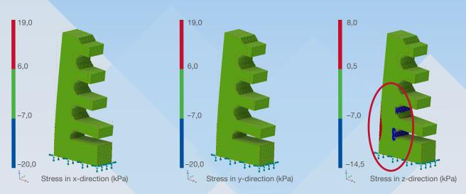
Fig 4: Brown Part Stability in each coordination direction \* Deformation is upscaled by a factor of 10 for illustrative purposes.
